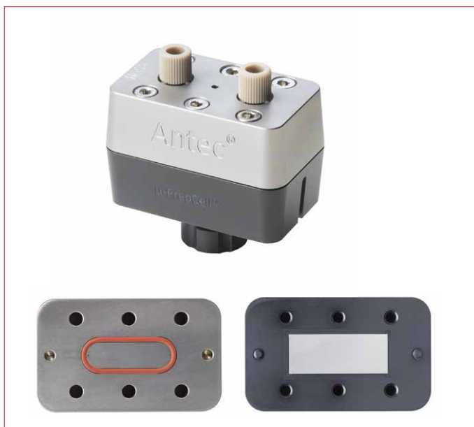
Figure 1: Ti inlet block used as active (working) electrode with sealing O-ring (left), rectangular Pt counter electrode in recess of black electrode holder (right)
